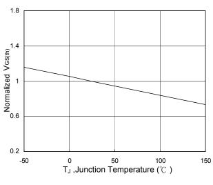
Fig.5 Normalized  $V_{GS(th)}$  vs. T<sub>J</sub>
