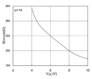
Fig.2 On-Resistance vs. Gate-Source
