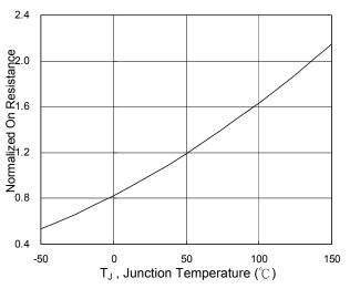
Fig.6 Normalized  $R_{\text{DSON}}$  vs.  $T_{\text{J}}$
