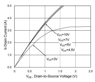
**Fig.1 Typical Output Characteristics**
