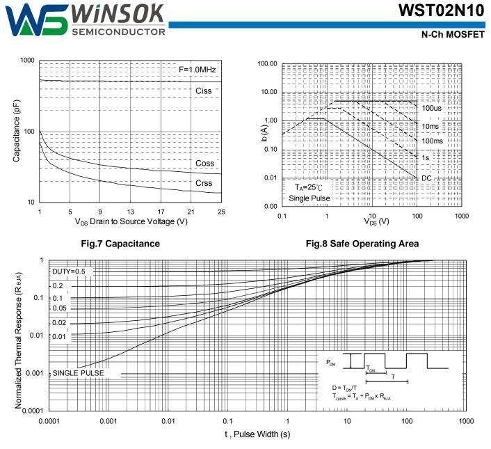
Fig.9 Normalized Maximum Transient Thermal Impedance
