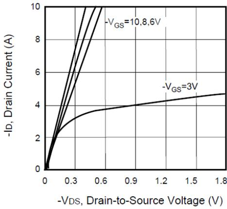
**Figure 1. Output Characteristics**
