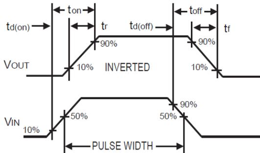
Figure 10. Switching Waveforms
