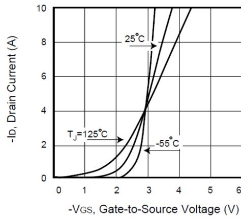
**Figure 2. Transfer Characteristics**
